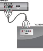
Video: Connect the remaining cables into the corresponding RGB (Red, Green, Blue) video output connections on the back of the converter box.
