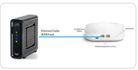
**Scenario 2:** Customer modem, eero, and Switch for additional Ethernet ports.
